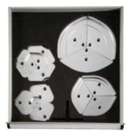
In order to efficiently clamp the raw material billets, special clamping jaws are mounted on to the steel body of the high-precision 3-jaw machine chuck. These sets of multi-range clamping jaws are made of high-grade aluminum and are designed to clamp certain diameter ranges of semi-finished billets.
